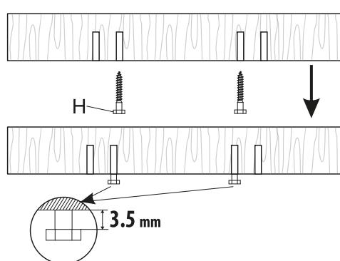
**EN:** Try the M8 x 60 screws marked (H) in the anchor in the hole. There can be a maximum distance of 3.5 mm between the plane of the ceiling and the screw head so that you can properly secure the bracket head.
