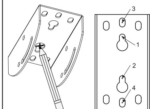
**EN:** After selecting the appropriate load-bearing location for mounting the bracket, place component (M1) on the ceiling and use a pen to select at least 4 mounting points. We recommend choosing the holes in the center of the console.
