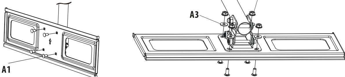
**EN:** Mount the rail (**M3**) to the end of the support rod (**M2**) using the 4 screws (**A1**), washer (**A2**) and nut (**A3**) provided. Make sure that the arrow on the front panel points up toward the support bar.
