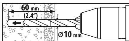
**EN:** Drill 6 holes according to the markings in which to insert the anchors marked with the letter (**I**) (10 x 50). Use a drill bit 10 for the operation, the depth of the hole should be 60 mm!
