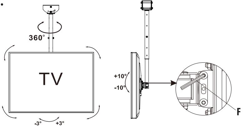
**EN:** You can adjust the angle of the TV by loosening and fixing the two allen screws on the back. The device can be rotated 360° after correct mounting. The manufacturer and distributor shall not be liable for any damage resulting from improper mounting.
