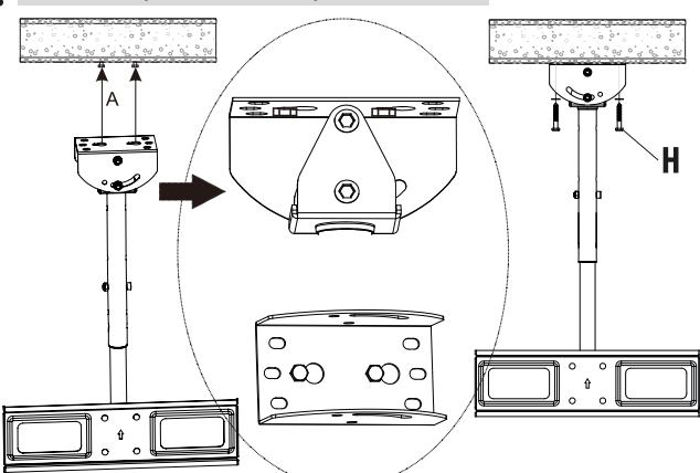
**EN:** Tighten all screws to secure everything. After checking all the screws, place the bracket head (**M1**) on the drilled 6 holes and secure it with the screws marked (**H**). Use a washer if necessary!
