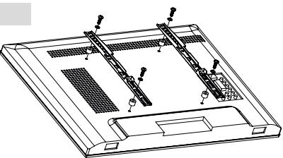
**EN:** Mount the two VESA-compliant mounting rails (**M4**) on the back of the TV. When mounting, use a spacer between the back of the TV and the rail (**G**) if necessary. Use the appropriate screw (**D / E**) and washer (**J**) for your TV to mount the rail.
