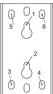
**EN:** After selecting the appropriate load-bearing location for mounting the bracket, place component (**M1**) on the ceiling and use a pen to select at least 6 mounting points. We recommend choosing 3-3 points per side.
